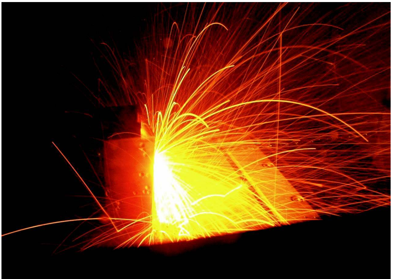
Elektronenstrahl-Schweißprozess an Dickblechen (40mm) aus Feinkornbaustahl Electron Beam Welding of thick plates (40mm) made of fine-grained structural steel
